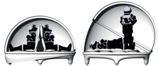
Sections: deployed shelter: minimal and maximal volume
