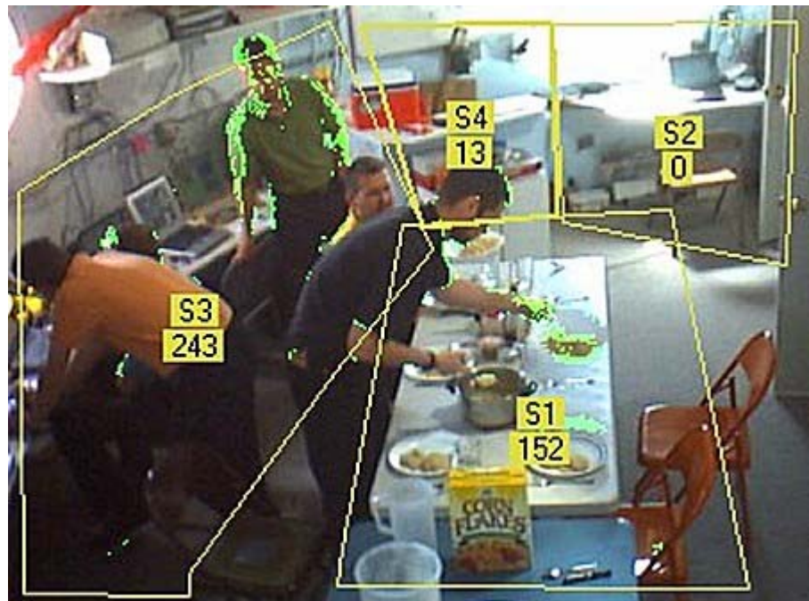
A screenshot from the object tracker software indicating areas of activities which will later be used to analyze workflow patterns.
