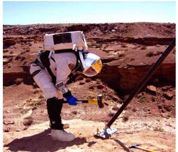
Securing the bi-ped rescue equipment into the soil can be a tedious task on a hard ground.
