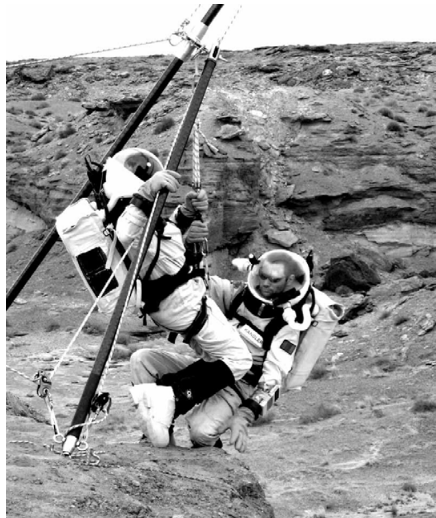
Fig. 3: The Health and Safety Officer (left) secures the IA (right) before tilting the Bipod to move him over the edge of the canyon.
