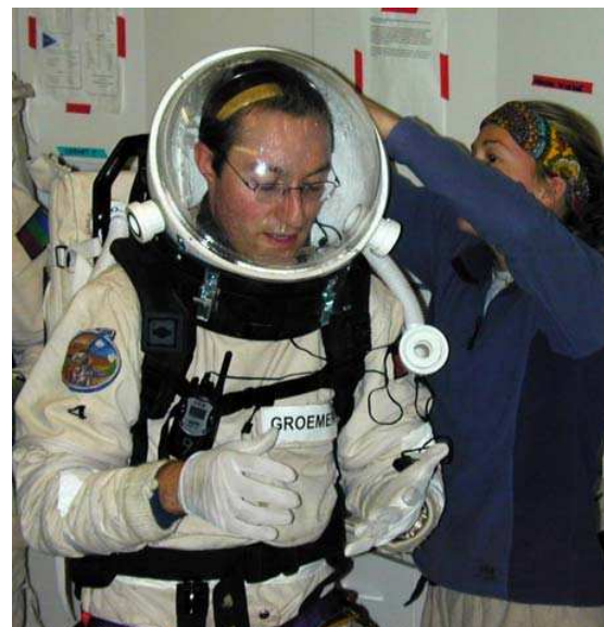
Fig. 5: Close-up of the simulated space suit of the US Mars Society with the personal life support system backpack (= PLSS). Note, that it takes an assistant to take off the life support rack. Undonning the suit during an emergency situation takes 15-20 minutes under AustroMars procedures
