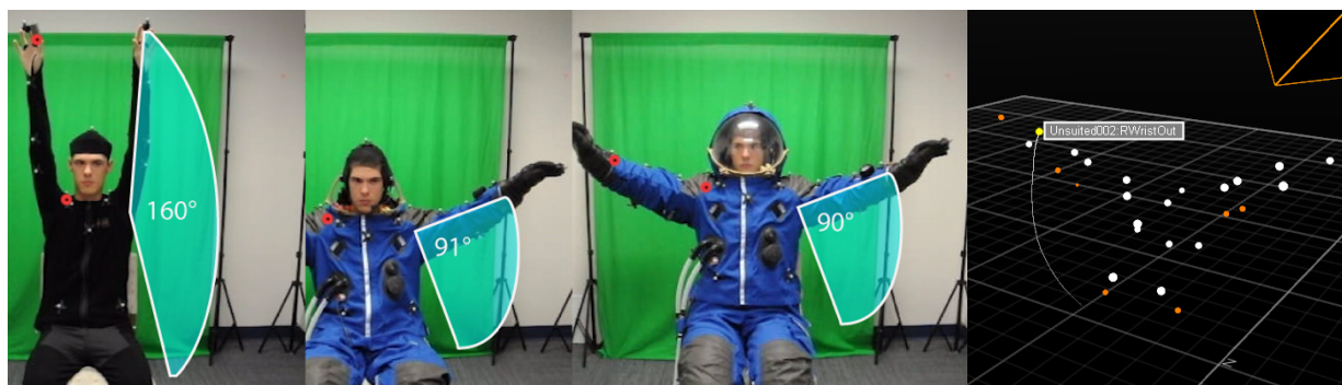
Figure 6: ERAU S.U.I.T Lab ROM Task B17 test with FFD's NASA Flight Opportunities Program spacesuit. Left: video capture shoulder angles in three test conditions. Right: OptiTrack 3D data of B17 suited motion.
