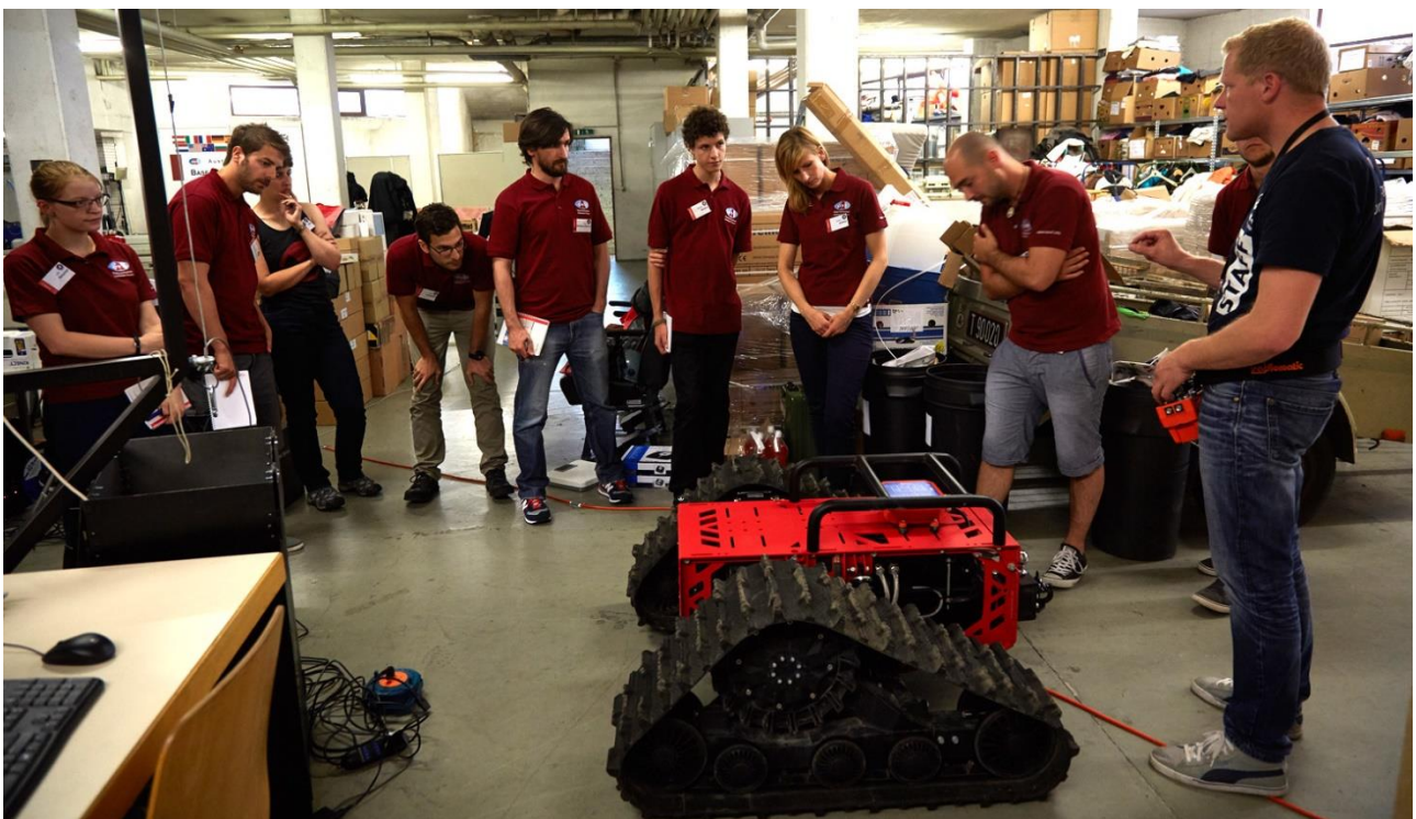
The Bock rover (provided by Mattro) was deployed for heavy-duty (up to 250 kg) cargo transportation in the field.
