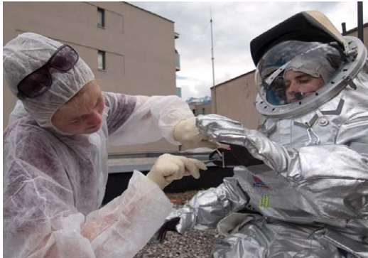
Figure 2: Swabbing test to detect microspherules contaminations on the Aouda.X spacesuit simulator (Photo taken during a training rehearsal, Credit: P. Santek)
