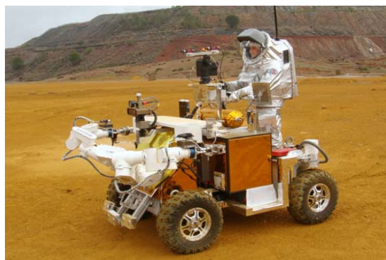
Figure 1: The Aouda.X spacesuit simulator and the ESA Eurobot Ground Prototype (Photo: OeWF/P.Santek)
