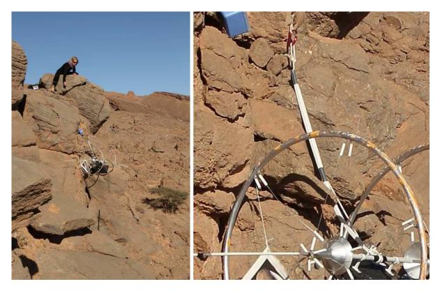
Vehicle blockage at the end of test 96: the anti yaw rod is engaged (and slightly bent) between two blocks. Under the vehicle (left photo) the black pole which will be used to push it upwards is visible.
