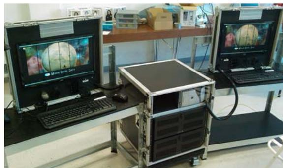
*OPS-BOX: The data hub for the field operations includes two work stations, plus a third in the OPS-SEAT White. The UPS allows for 30min of operation without the main power supply.*
