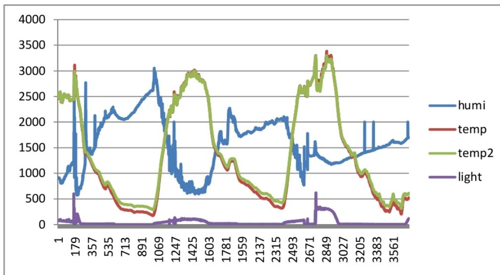
fig. 8. Data sets retrieved from one of the MOTs (the little blue boxes/mobile sensors). The data spans from 04-02-2013 14:37 until 07-02-2013 07:01. The measurements were taken in every minutes.
