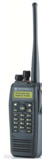
The radios used in the field were based upon 8 units Motorola DP3601, with a Mototrbo base station. The exact frequencies were allocated by the Moroccan ANRT (Agence Nationale de Réglementation des Télécommunications).
