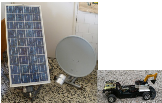
Figure 6. The solar panel and the dish for radio communication, and the sample collecting rover.
