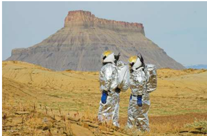
Fig. 3: BioMars sterile suits composed of Mylar-foil were used to track backward contamination under various exploration scenarios.
