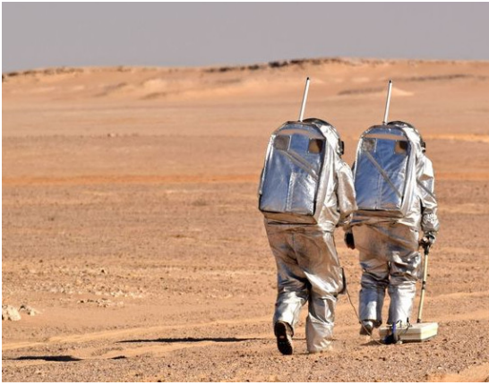
Figure 2: The analog astronauts during ScanMars experiment data acquisition. The radar sledge is being pulled along the planned profile.
