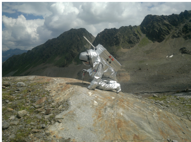
Figure 4. Fully-suited analogue astronaut taking SHRT measurements on glacially abraded bedrock (polygon no. 12). Source: Taken by the M. Dąbski.
